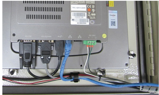
Ethernet connections to the TT-TS12 are made with a standard RJ-45 connector to either of two network ports on the rear side of the touch screen computer at the base
