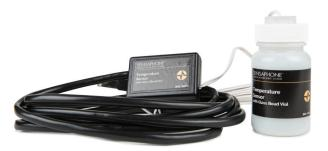
This sensor is designed to connect to the Sensaphone IMS series product line. The glass bead filled vial will buffer any momentary fluctuations that may cause a preliminary alarm such as defrost cycles, opening of doors and fans circulating air. The glass beads will slow the response time of the sensor allowing normal daily operations to occur without having an alarm initiated. The sensor can reliably monitor temperatures as low as -122°F (-86°C).
