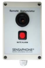
The Sensaphone FGD-0088 Remote Annunciator is a 12-24 Volt 90 decibel alarm buzzer in an enclosure. It can be used in conjunction with many other devices as a local alarm or as a remote alarm. This provides flexible monitoring via audible and visual alert whenever an alarm exists.
